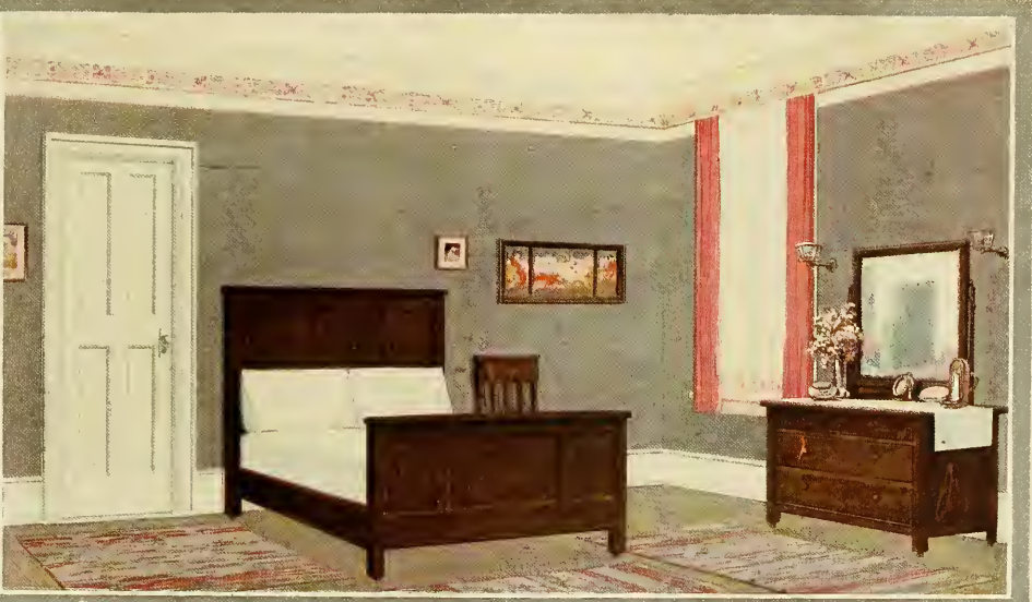
Specification— Ceiling and Drop , S-W Flat-tone, White. Wall , S-W Flat-tone, French Gray. Stencil , No. 18y. Woodwork , S-W White Enamel. Floor , S-W Inside Floor Paint, Gray.
